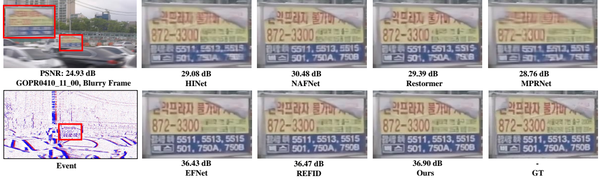
Figure 5: Qualitative comparison results of different image deblurring methods on the GoPro dataset.
