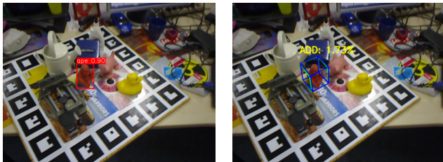
Figure 4. Qualitative results of YOLOv10m object detection (left) and the final 6D pose estimation of the detected object (right).
