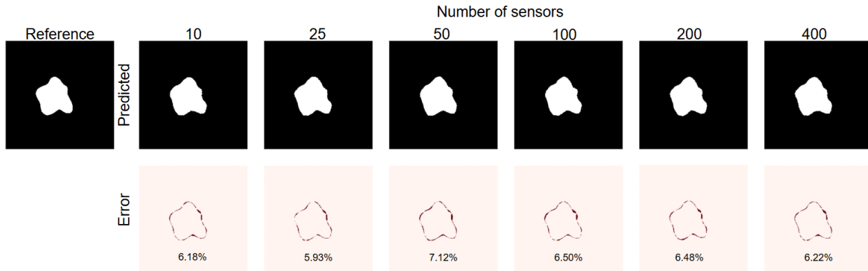
Figure 12. Ablation of the number of sensors on Helmholtz inversion.
