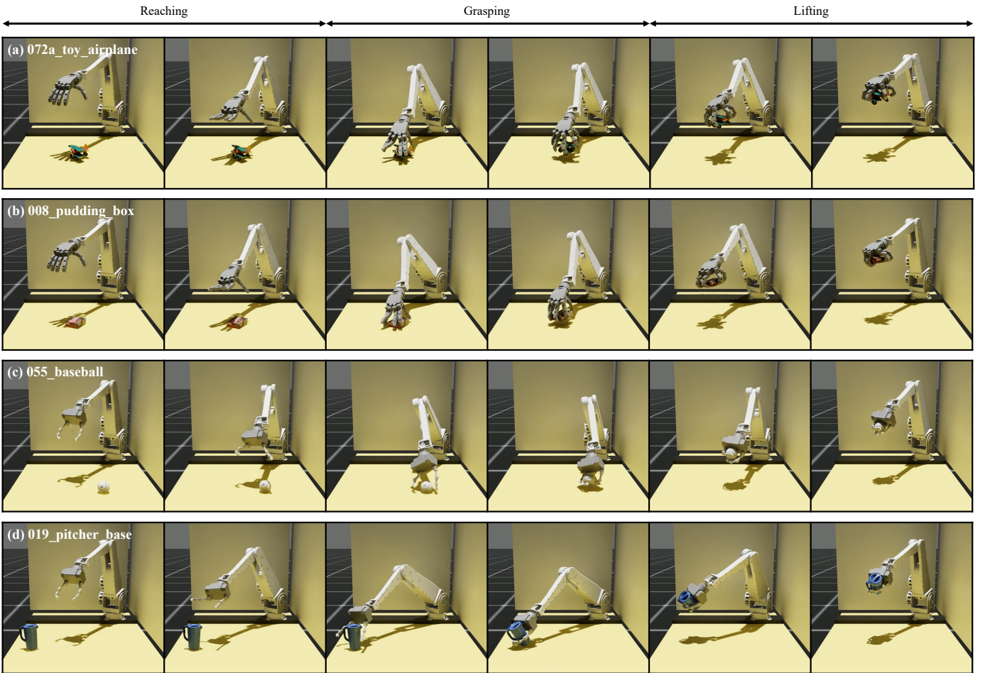
Fig. 4: Simulation results demonstrating the reach-grasp-lift progression of the proposed framework. The top two rows show the 20-DoF 5F hand grasping (a) a toy airplane (ID: 072a) and (b) a pudding box (ID: 008). The bottom two rows show the 8-DoF 2F gripper grasping (c) a baseball (ID: 055) and (d) a pitcher base (ID: 019). Our proposed control framework successfully generalizes diverse grasping strategies to various geometries across various end-effector platforms, demonstrating its robustness and adaptability in dexterous grasping tasks.
