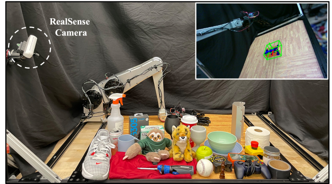
Fig. 7: Experimental setup for real-world hardware validation. We evaluated our policy on 26 diverse objects. A RealSense camera (top left) computes the object state in real time. The top-right inset shows the camera’s perspective, extracting the target object state used as the observation for the RL planner. The manipulator platform is located in the left rear corner.
