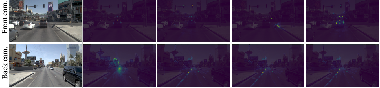
Figure 5. Attention maps of scene tokens. From the final attention layer, front-camera tokens specialize to distinct regions (traffic light, lead vehicle, road edges), while back-camera tokens largely collapse to the same features, aside from a single distinct token.
