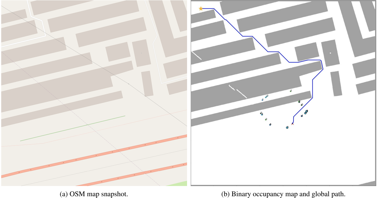
Figure 3: Example of map processing: (a) an OSM map snapshot from which occupancy maps were formed; (b) the corresponding binary occupancy map with a global path constructed using A*.
