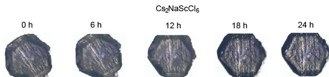
Figure S21. Humidity stability tests (100% RH, 25°C) from 0 to 24 h. Optical microscope images of \text{Cs}_2\text{NaScCl}_6 single crystals.
