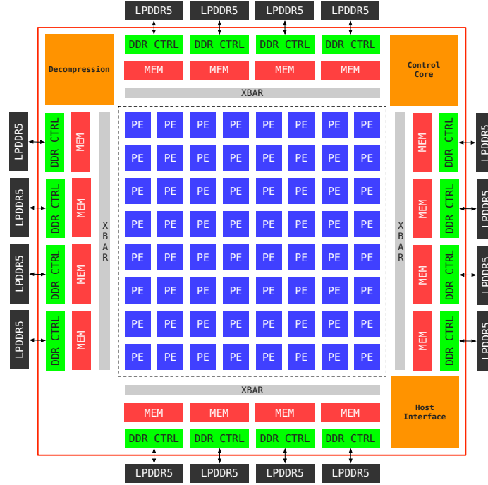
Figure 7 MTIA 2i architecture featuring an 8×8 processing element (PE) array interconnected via network-on-chip. Each PE contains dual RISC-V cores and specialized fixed-function units: Memory Layout Unit (MLU) for data transformation, Dot Product Engine (DPE) for matrix operations, Reduction Engine (RE) for aggregations, SIMD Engine (SE) for vector operations, and Command Processor (CP) for control flow (more details can be found in Section 3 of [Coburn et al. (2025)]).
