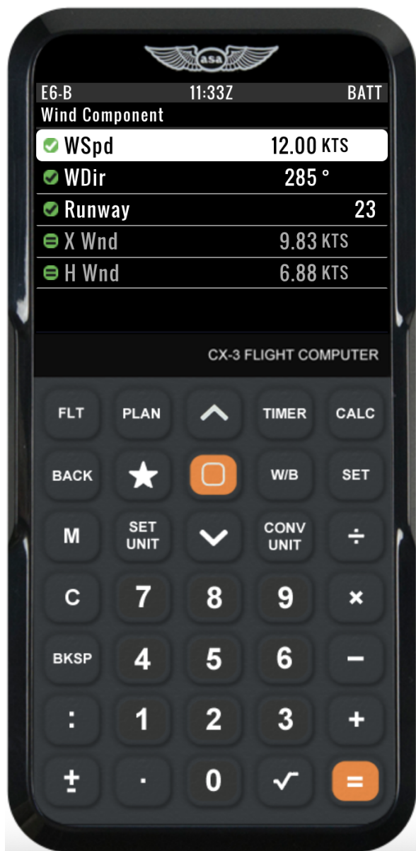
(a) Wind components calculated by a traditional electronic flight calculator (ASA CX-3). The device reports numeric headwind and crosswind components only, without visual context or explanatory support.
