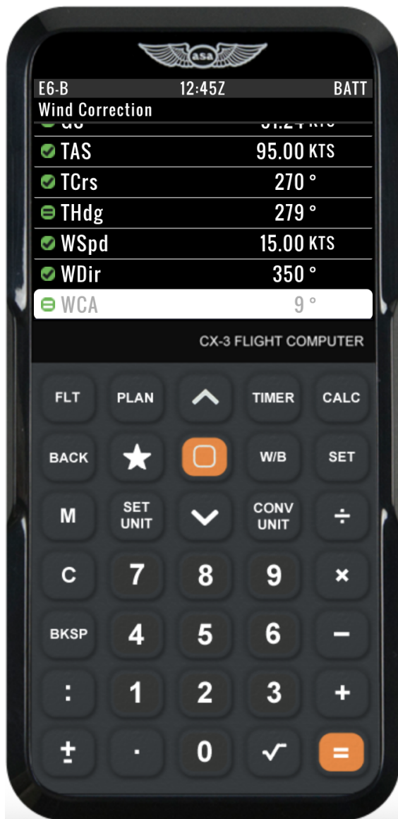
(a) Wind correction angle (WCA) calculated by a traditional electronic flight calculator (ASA CX-3). The device reports numeric wind correction and ground speed values only, without visualisation of wind vectors or spatial context.
