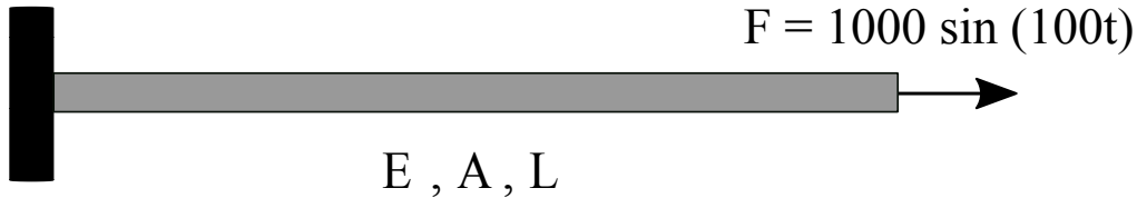
Figure 9: Cantilever beam with a sinusoidal forcing at the end
