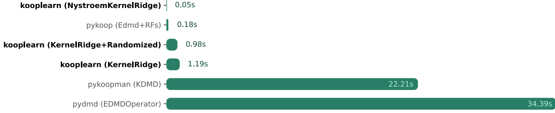
Figure 3: Fit time of a Kernel model (Gaussian kernel) on a dataset of 5000 observations from the Lorenz 63 dynamical system. The results are the median of three independent runs on a system equipped with an Intel Core i9-9900X CPU (3.50GHz) and 48GB of RAM memory.
