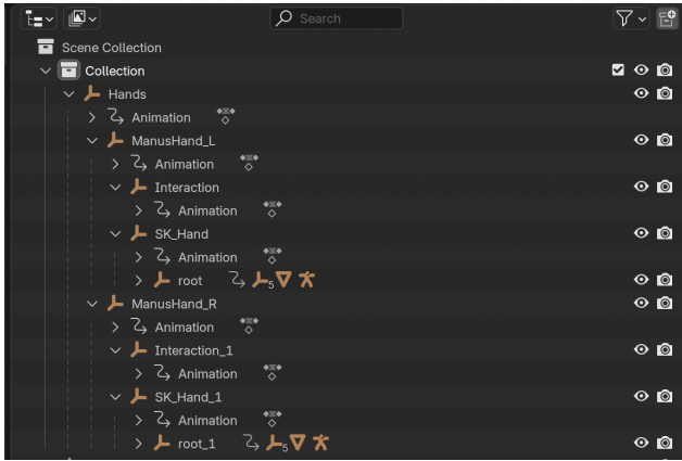
Figure S4. FBX hierarchy from the MANUS export. Hands controls global placement. ManusHand_L and ManusHand_R parent the SK_Hand meshes and a per-hand root armature with finger and thumb mocap. Animation and Interaction store non-finger transforms that we remove for retargeting.
