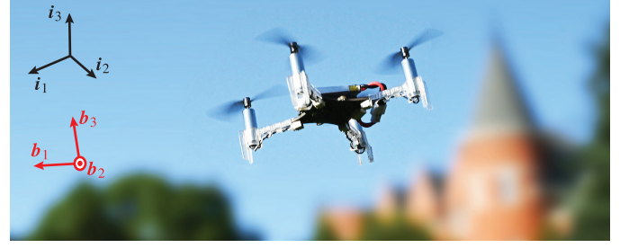
Fig. 1. Picture of the UAV used in the flight control experiments. The Crazyflie 2.1 quadrotor and the definitions of the inertial frame of reference, \mathcal{I} = \{\mathbf{i}_1, \mathbf{i}_2, \mathbf{i}_3\} , fixed to the planet and the body-fixed frame of reference, \mathcal{B} = \{\mathbf{b}_1, \mathbf{b}_2, \mathbf{b}_3\} (shifted for clarity), whose origin is attached to the center of mass of the robot.
