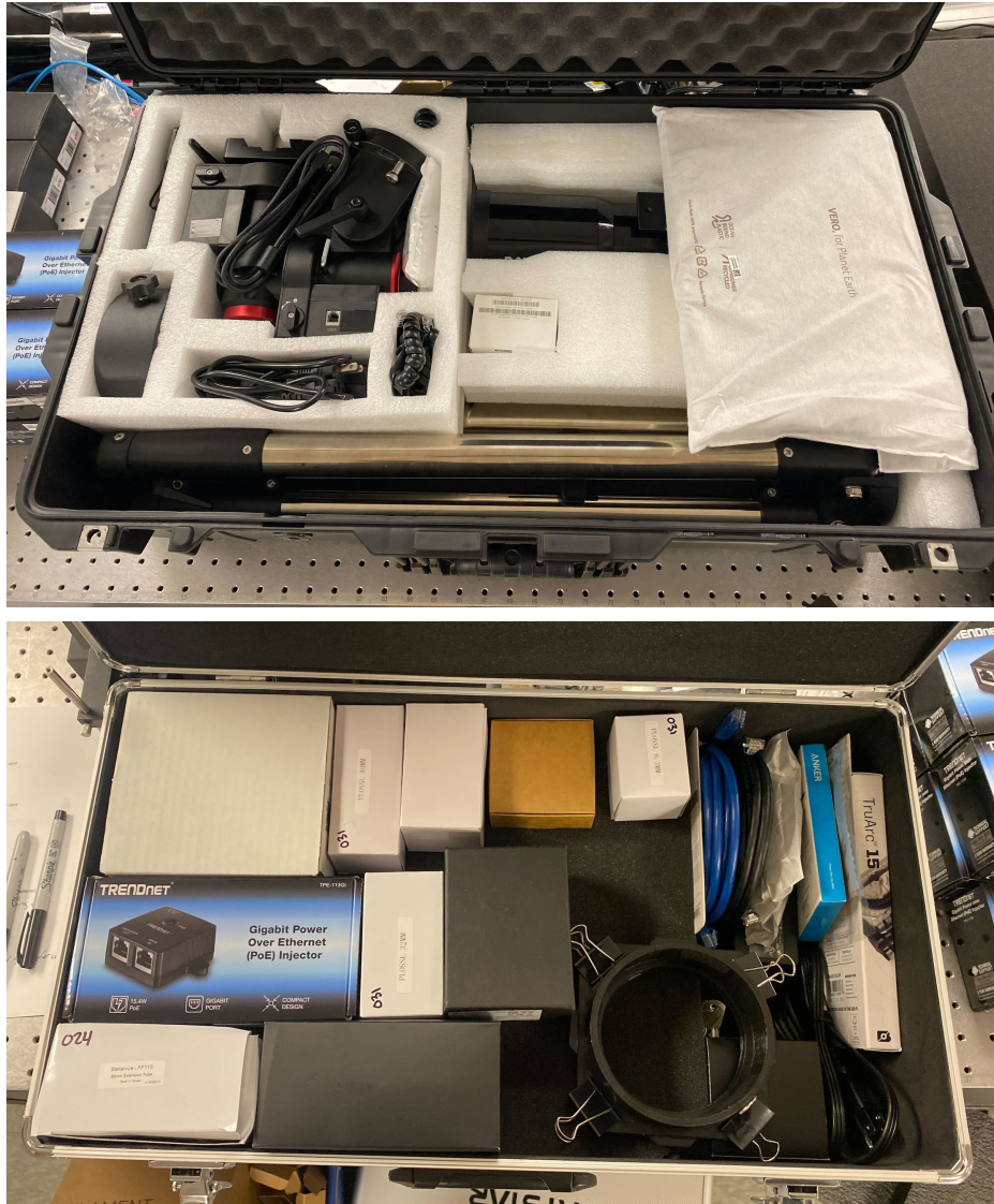
Figure 5. Example of how equipment was packaged prior to shipment. (Top) Pelican Air 1615 housing the telescope, mount, tripod, camera, and laptop. (Bottom) Daystar case housing all supplemental equipment that did not fit into the Pelican case.
