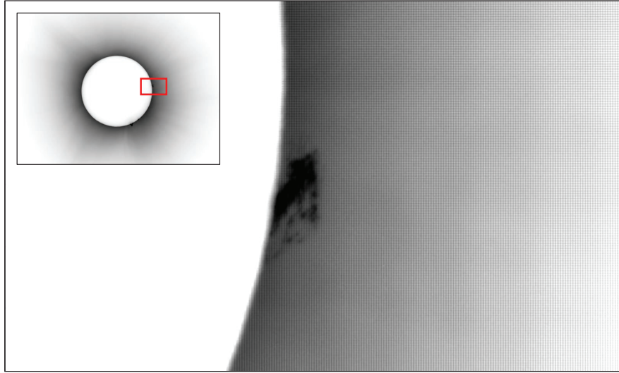
Figure 11. HDR image from Site 034 (UTC 19:33:23) displayed with an inverse color table. The inset image is the full field of view, while the large image emphasizes “crosshatch” of the individual polarizers within the macropixels of the region of interest outlined in red.
