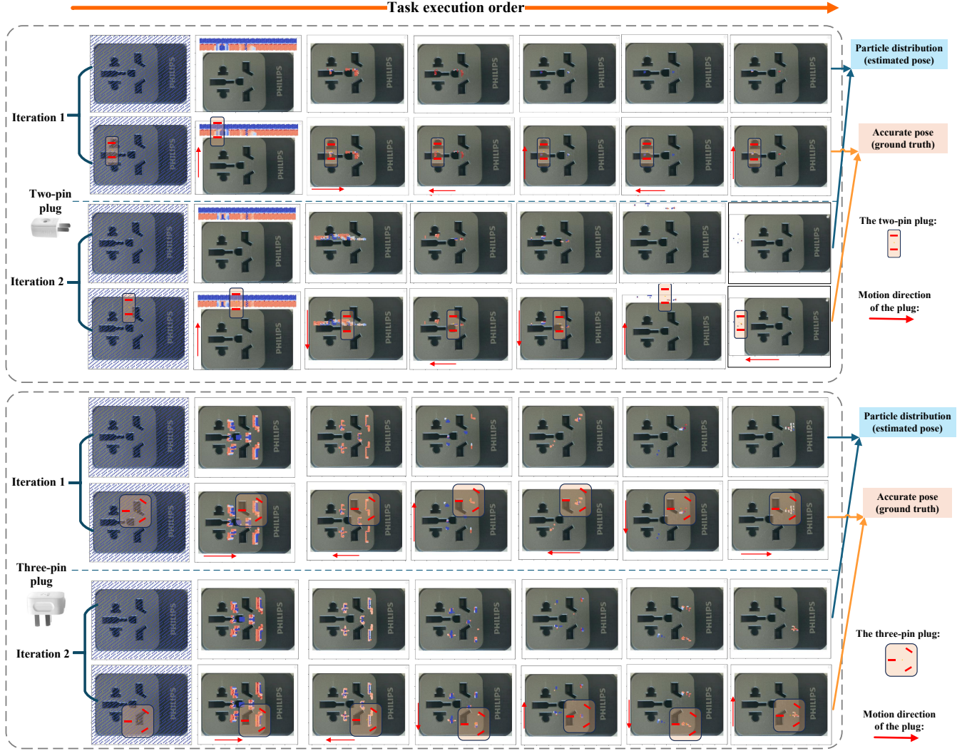
Fig. 6. The results of socket assembly experiments in different initial locations. The distribution of particles represents the potential relative pose of the plug and the socket. Red particles represent that the plug could be located at this point with more possibility, while the blue particles represent the less possibility.
