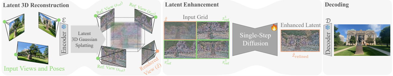
Figure 2. Framework Overview. Given a set of input views with known camera parameters, each image is encoded into the VAE latent space of a diffusion model. We then perform 3DGS optimization to reconstruct the underlying latent radiance field. Due to multi-view inconsistencies in diffusion VAEs latent space, a rendered novel view latent lacks high frequency details. We tile this rendered view together with reference views into a grid, and leverage a single-step diffusion model with self-attention mechanism that aggregates information across all views. The enhanced latent image is finally decoded to receive the novel view image.
