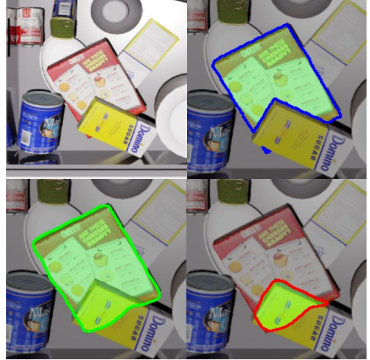
Fig. 1. Sample of ViTA-SimData (top-left), visible mask (top-right), predicted amodal (bottom-left) and occluded mask (bottom-right) of ViTA-Seg Dual Head.
