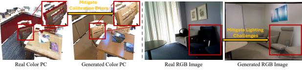
Figure 6. Our Match-ControlNet effectively mitigates calibration errors and lighting challenges commonly encountered in real-world RGB-D data, thereby improving the matching precision of color point cloud registration methods.
