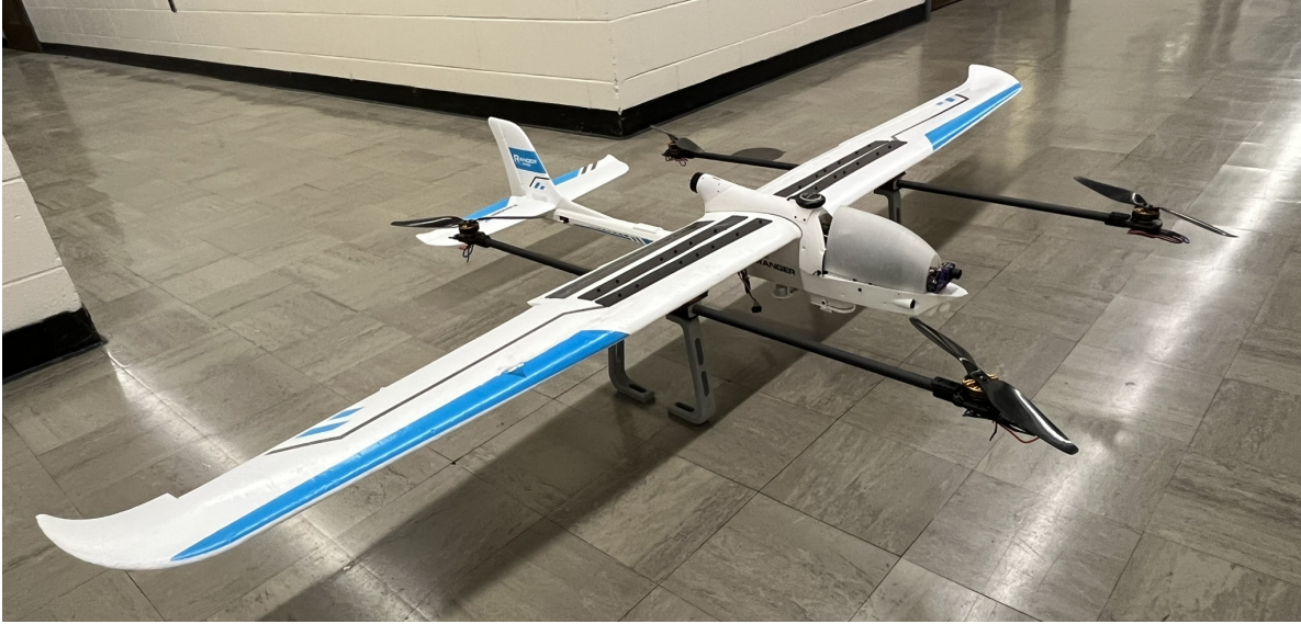
Fig. 1 QuadPlane prototype featuring RGB, RGBD (Intel Realsense), FPV Cameras and Jetson Orin Nano
