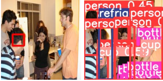
(a) Original image with a partition in the 5 \times 5 partition scheme highlighted. (b) YOLO detections on the original image.
