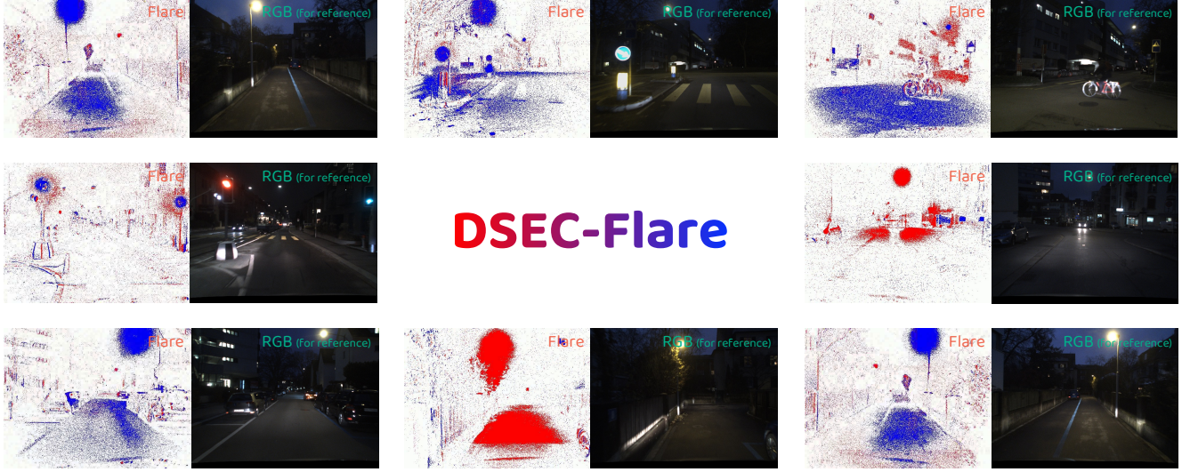
Figure 10. Examples from DSEC-Flare. This is a real-world dataset that showcases typical lens flares induced by various light sources. For each example, we show the raw event stream and a corresponding RGB image to illustrate the light sources causing the artifacts. Best viewed in colors and zoomed-in for details.
