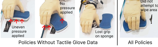
Fig. 7: (A) Real robot policy rollouts with the Psyonic Ability Hand and Franka robot arm. (B) Failure modes for policies with and without tactile feedback.
