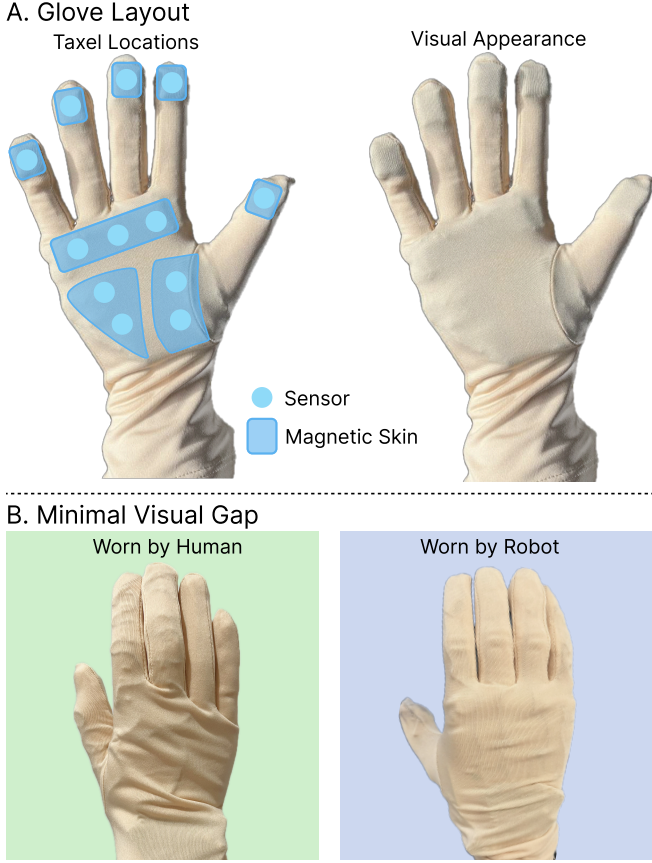
Fig. 5: A) Glove layout maximizing sensing coverage while minimizing encumbrance. B) The shared glove platform minimizes the visual gap between the human and robot hand.
