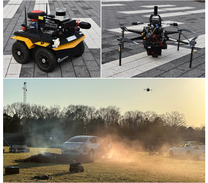
Fig. 1: Our heterogeneous robot team for triage during a mass casualty simulation at the Guardian Centers, Perry, GA in March 2025.
