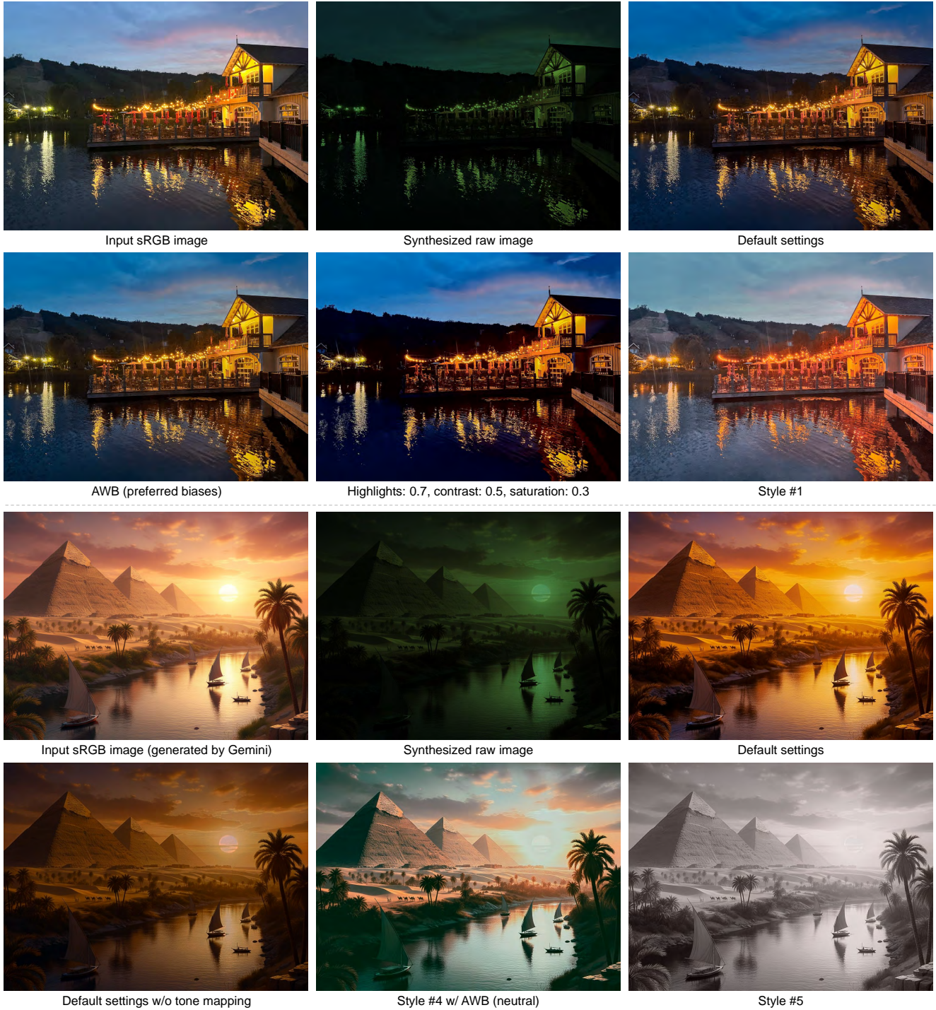
Figure 33. To broaden the applicability of our tool to sRGB images saved without embedded raw data (i.e., outside our framework), we linearize the input sRGB images (whether produced by unknown ISPs or generated by AI models) into synthetic raw-like representations, thereby enabling the full functionality of our pipeline. The top example shows an image captured and rendered by the iPhone camera ISP, from which we generate a raw-like image and process it with different settings using our tool. The second example is an image generated by the Gemini 2.5 Flash Image model with the prompt: Generate an ancient Egyptian scene with pyramids, the Nile, and palm trees glowing under a golden sunset. We convert it into a raw-like image and apply our tool with different rendering options.
