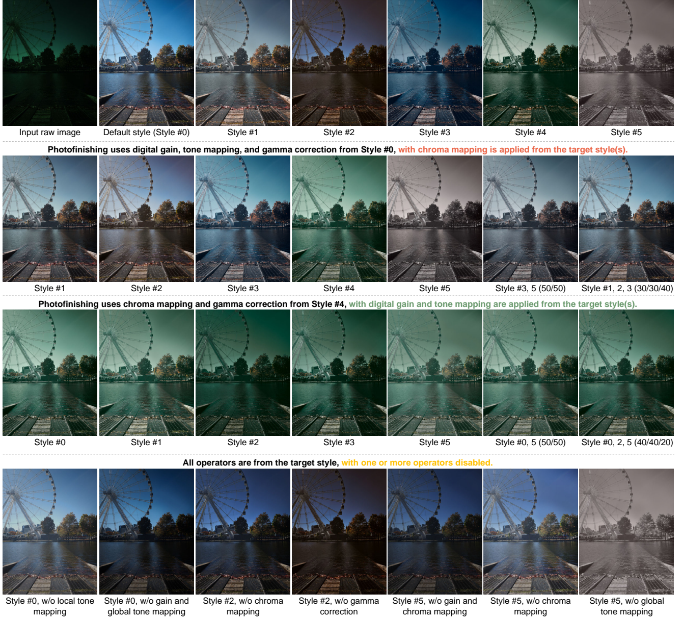
Figure 31. Our modular photofinishing design provides users with full control over the picture style of the final image. In addition to selecting from pre-defined picture styles (each rendered by a pre-trained photofinishing module), users can also mix operators from different styles or disable specific operators entirely. The shown example was captured with the iPhone 13 main camera, which is an unseen camera for our pre-trained photofinishing modules.
