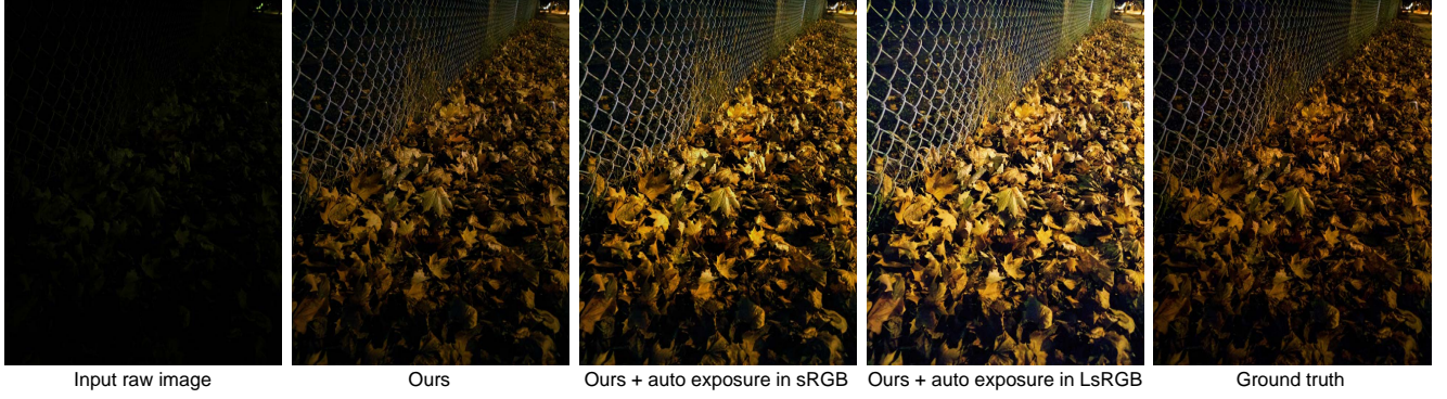
Figure 25. We allow applying auto exposure (AE) after conversion to linear sRGB and directly before the photofinishing module. This figure shows a qualitative example from the S24 validation set [16], including the input raw image, our output without AE, and with AE applied either at the end of the pipeline or in linear sRGB. The ground-truth sRGB image from the S24 dataset is shown for reference.
