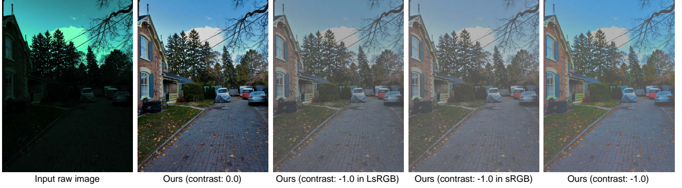
Figure 27. We implement a user-controlled contrast adjustment on the luminance channel after local tone mapping. This figure shows a qualitative example from the S24 validation set [16], including the input raw image, our output without adjustment ( \alpha_{\text{contrast}} = 0.0 ), and with reduced contrast ( \alpha_{\text{contrast}} = -1.0 ). For comparison, results are shown when the adjustment is applied after local tone mapping in linear sRGB, after the full photofinishing module, and to the Y channel after local tone mapping ( \mathbf{Y}_{\text{LTM}} ) in YCbCr (our choice).
