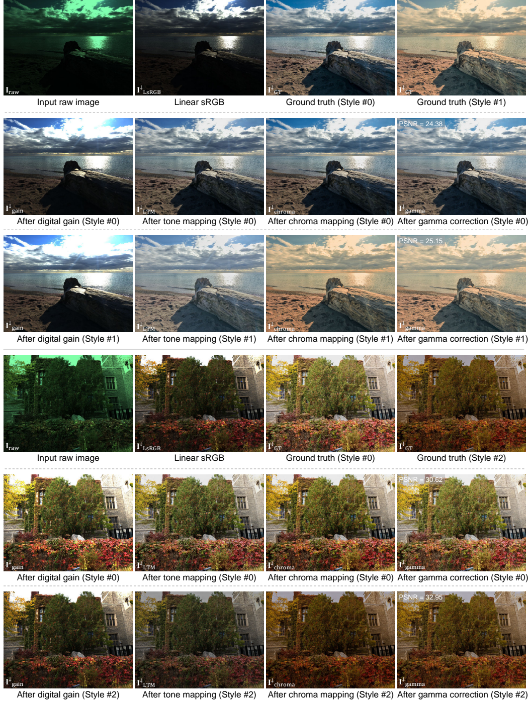
Figure 47. Comparison of intermediate-stage outputs for the same scene rendered with different picture styles. Images are taken from the S24 test set [16]. The examples illustrate how the photofinishing stages adapt their tone and chroma adjustments depending on the target picture style.
