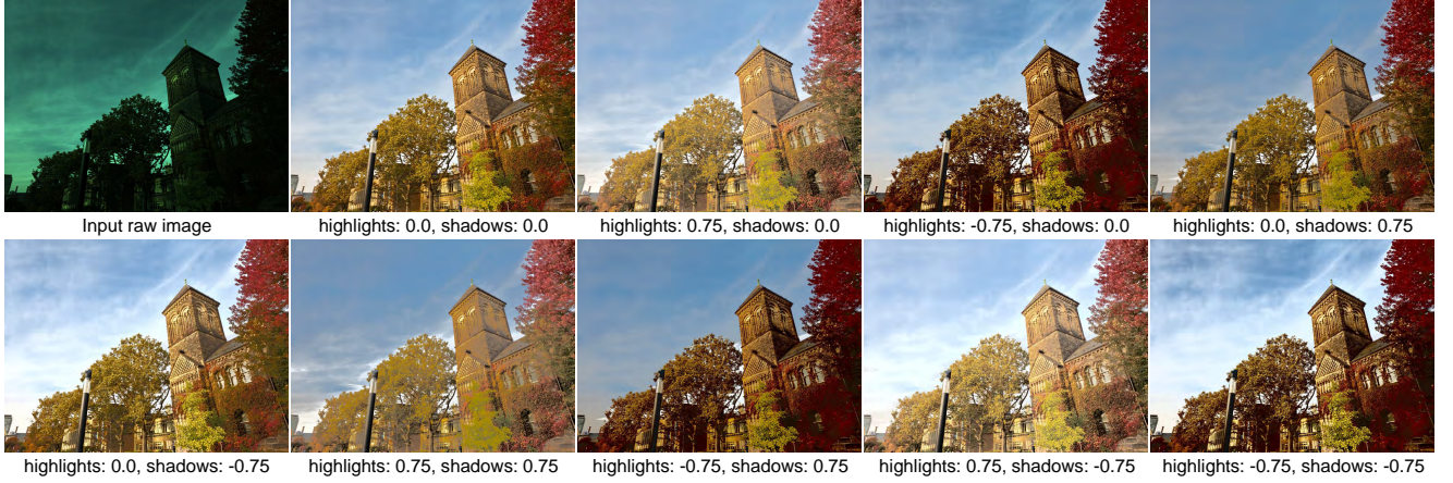
Figure 28. We allow the user to optionally adjust highlights and shadows after applying local tone mapping. Shown here is an example from the S24 validation set [16], including the input raw image and our outputs with different values of the highlight and shadow control parameters, \alpha_{\text{high}} and \alpha_{\text{shad}} , respectively.
