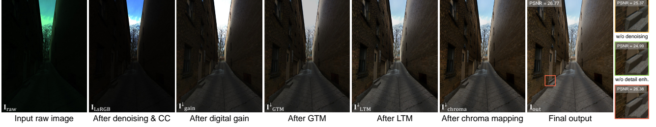
Figure 44. Outputs of the intermediate stages in our pipeline, including raw denoising, color correction (CC), and the photofinishing module, which comprises digital gain, global tone mapping (GTM), local tone mapping (LTM), chroma mapping, and detail enhancement (enh.). We show enlarged patches of the final result when raw denoising is disabled, when detail enhancement is disabled, and when both are enabled. The example is taken from the S24 test set [16].
