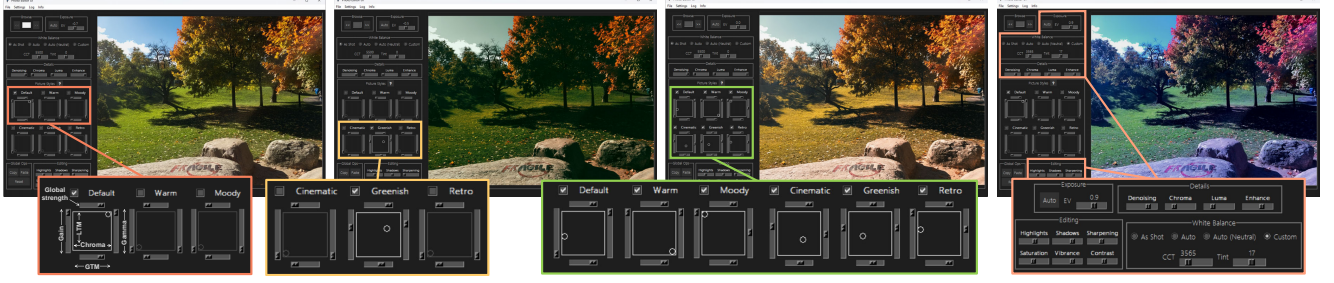
Figure 3. User-interactive photo-editing tool built on our modular ISP, providing full control over the rendering process, picture styles, and editing options. The interface supports selecting or interpolating between styles and adjusting white balance, exposure, color, and overall appearance. See the supplementary material (Sec. I) and the video (click to view) for details.
