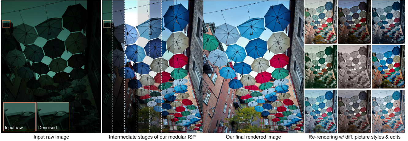
Figure 1. We present a modular neural image signal processing (ISP) framework that offers full control over every stage of the pipeline and can handle unseen cameras without requiring re-training. On top of this framework, we built a user-interactive tool that supports post-editable re-rendering, allowing users to re-process saved outputs with different picture styles and manual adjustments. The shown image was captured in raw format using the iPhone 13 main camera, then denoised and processed by our modular ISP, with intermediate stages and multiple picture-style and manual-adjustment results displayed. None of our models were trained on data from iPhone cameras.
