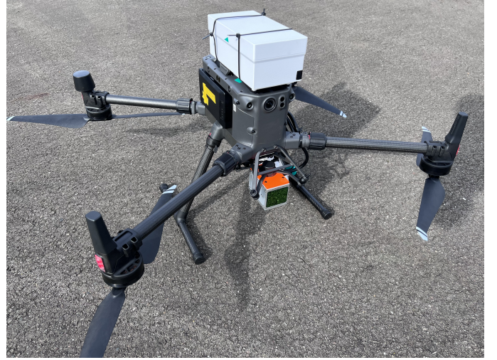
Fig. 4: Livox Avia mounted below a DJI M300 RTK drone, with embedded computer system mounted on top.
