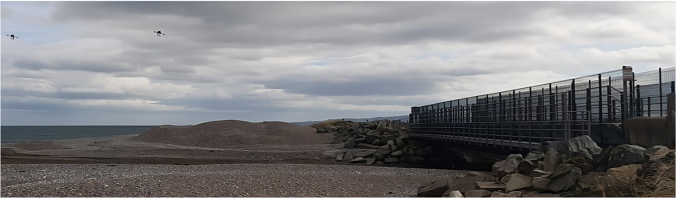
Fig. 1: Two DJI M300 RTK drones midflight (top left), with railway bridge (right). The left-most drone is equipped with a Zenmuse L1 LiDAR. The drone to its right is equipped with the Zenmuse P1 photogrammetry camera.
