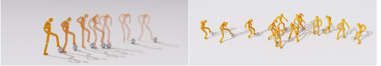
Figure 5. Visualization of synthesized ball-dribbling motions using our hierarchical controller. Our framework learns diverse skills from 2D motion data, exhibits natural transitions between different dribbling styles (left), and demonstrates seamless composition and switching between directional movements.
