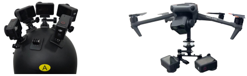
Figure 3. Left: Our 5 DJI Action 5 Pro camera helmet rig. Right: Our two synchronized DJI Action 5 Pro on DJI Mavic 3 Pro drone.
