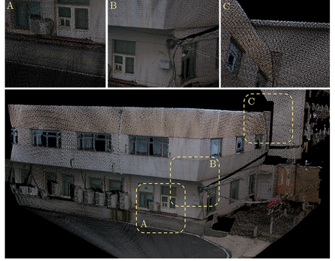
Fig. 1. Colorized LiDAR points by camera RGB image with calibrated extrinsic parameters using the proposed method. The second row is the overall color point cloud, and the first row is the enlarged picture of the local details in the color point cloud.
