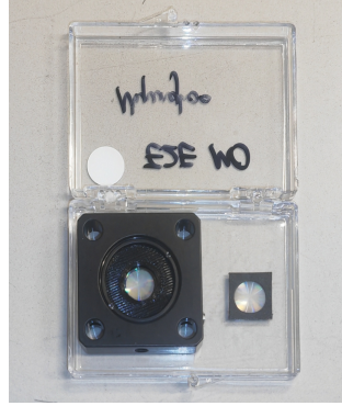
Figure S1: Images of our end-to-end lens(right) and hyperboloid(left) lens used for experiment. Their apertures are designed to be identically 1cm
