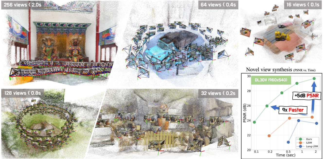
Figure 1. Our method efficiently processes a wide range of input views, reconstructing diverse large-scale scenes in under 0.1–2.0 seconds. We utilize Viser [73] for 3D scene visualization. Each marker in the plot represents performance under different numbers of input views: 16, 32, 64, 128, and 256 views for Ours, and 16, 32, and 64 views for both iLRM and Long-LRM. See Tab. 9 and 10 for further details.
