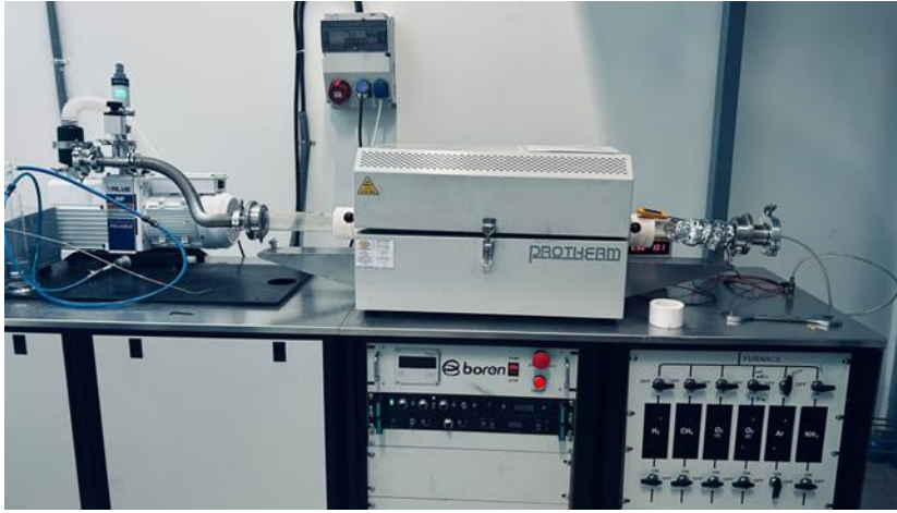
Fig.1. LPCVD system for the h-BN growth.
