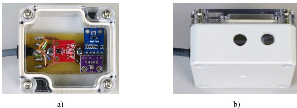
Figure 4a, b. Mounting sensors on a printed circuit board and installing the printed circuit board with sensors in a mounting box featuring a transparent top cover (a). View of the drilled holes from the side of the box (b).
