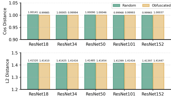
Figure 3: The statistic comparison between Amulet obfuscated weights vs. original weights and random matrices vs. original weights.
