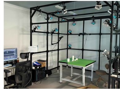
Figure 3: Motion capture system configuration showing optical marker placement and capture volume.
