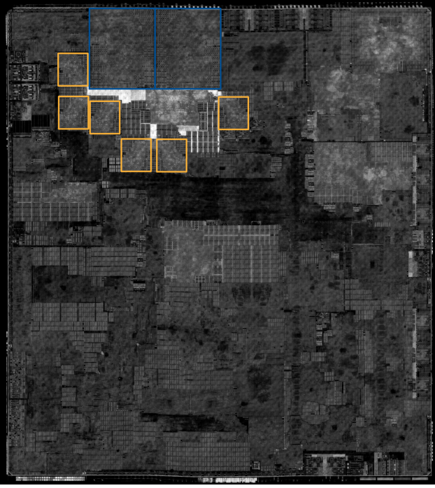
Figure 12: IR die-shot of the Snapdragon 750G 5G SoC. The two ARM Cortex-A77 cores are outlined in blue, the six ARM Cortex-A55 cores are marked with yellow rectangles.
