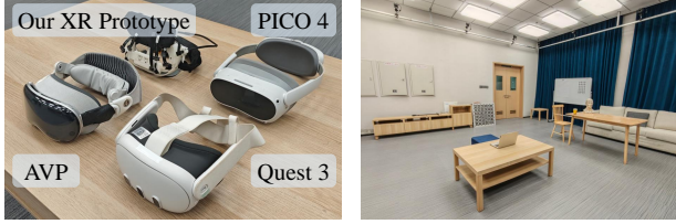
Fig. 10: DUTs for SLAM benchmarking (left) and the test environment (right). The DUTs include AVP, Quest 3, and PICO 4. Additionally, our XR prototype is used for collecting the SLAM sensor data as the inputs to open-source SLAM algorithms.
