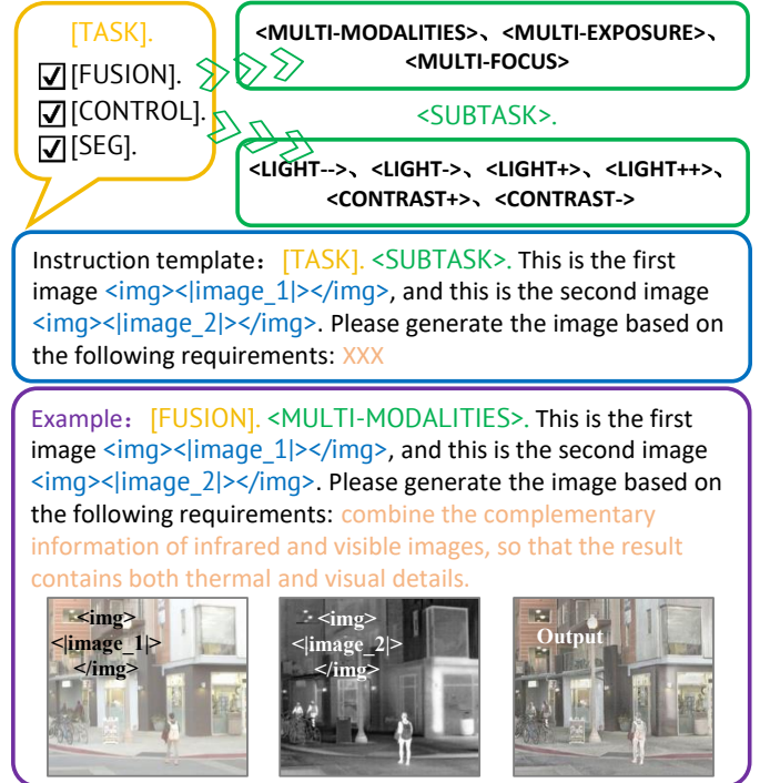
Fig. 6: Illustration of the prompt structure. Each prompt consists of four components: a [TASK] tag, a <SUBTASK> tag, two image placeholders <img><image_n></img>, and a free-form textual instruction. For fusion tasks, the tag is [FUSION] with subtags <MULTI-MODALITIES>, <MULTI-EXPOSURE>, or <MULTI-FOCUS>. For image control tasks, the tag is [CONTROL] with one of the subtags <LIGHT++>, <LIGHT+>, <LIGHT->, <LIGHT-->, <CONTRAST+>, or <CONTRAST->. Segmentation tasks use the tag [SEG] without a subtask. For M3 data, only the general tag [FUSION] is used, without any subtask tag.
