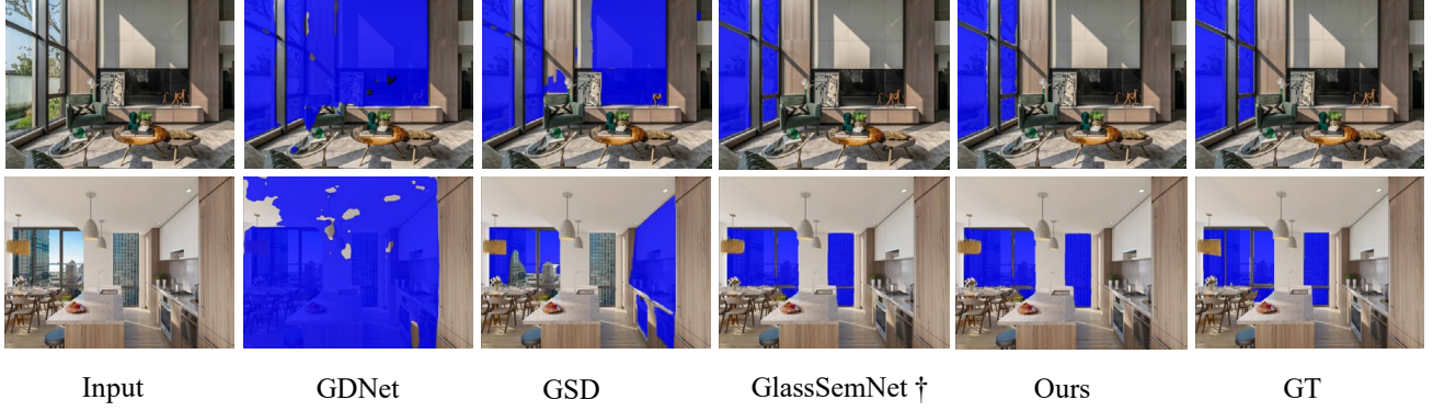
Figure 10. Qualitative comparison of our method with other methods on GSD-S dataset [36]. (†) denotes the glass segmentation method with semantic context and post-processing refinement.
