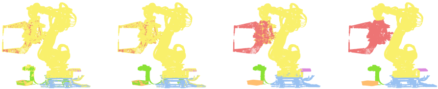
Figure 5: 3D point cloud segmentation results. From left to right: (a) Projection-only (b) With cluster method (c) With Bayes (d) GT
