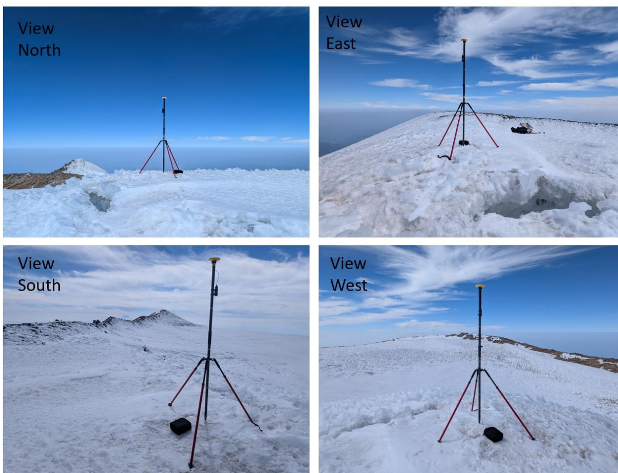
Figure 6. The GNSS mounted on Columbia Crest. Views look North, East, South, and West.
