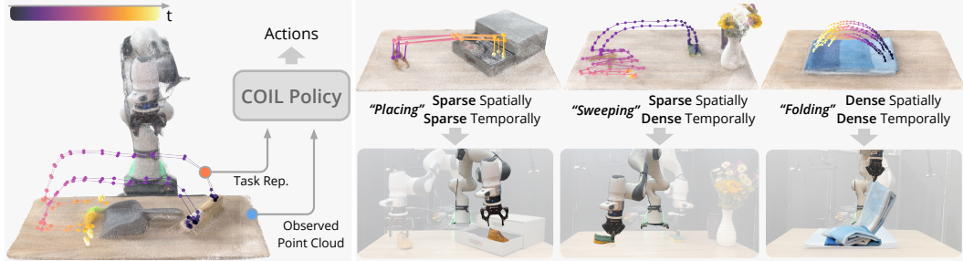
Figure 1: We introduce COIL , an approach for versatile manipulation conditioned on a correspondence-oriented task representation in 3D. Each task is defined by a set of keypoints annotated on the observed point cloud of scene objects, with task goals and constraints expressed as their intended 3D trajectories. Unlike prior work that assumes a fixed number of keypoints or densely sampled time steps, COIL supports task specifications with variable spatial and temporal granularity, allowing users or planners to adapt the level of detail based on the task’s complexity or intent.
