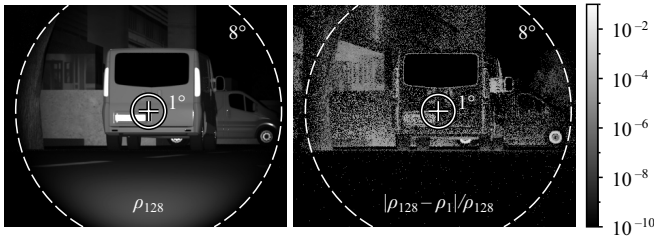
Fig. 7: Deviations between the proposed single-bounce intensities for \rho_1 and a full computation of 128 bounces \rho_{128} (each 128 samples/px) using the Cycles raytracer for a single beam with an extreme radius of 8^\circ . Intensity differences are around 10^{-2} on the rough steel wheels, mostly however below 10^{-4} .
