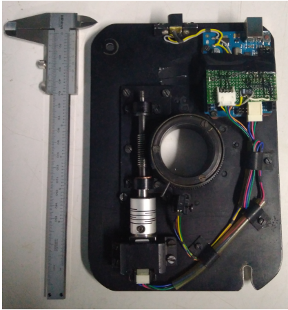
Fig. 3: Half-wave plate and its control unit.
