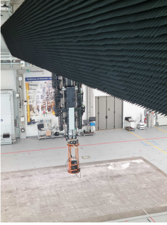
Fig. 9: 3D positioning system with mounted setup in the test station.
