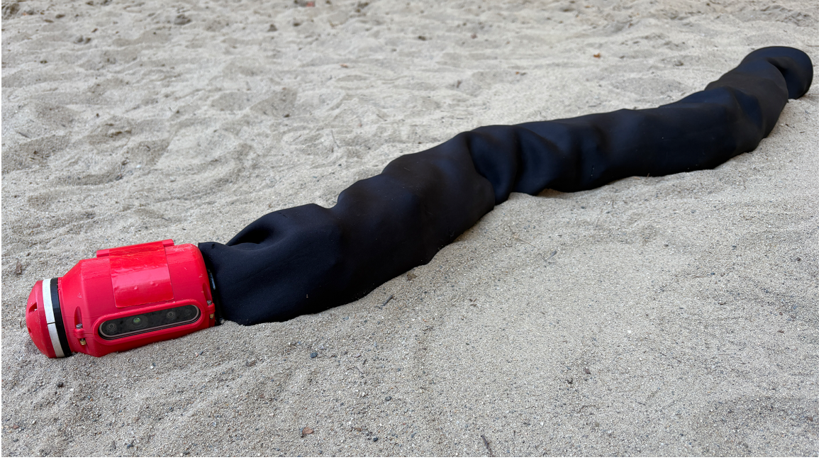
Figure 1.1: COBRA robot performing sidewinding motion across loose sandy terrain.
