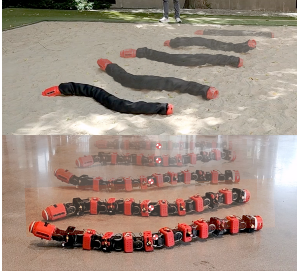
Figure 3.5: Snapshots of the snake robot operating in rigid laboratory conditions using motion capture and on loose outdoor sand using onboard visual–inertial odometry. Both setups are used to benchmark the predicted behavior from rigid and deformable terrain simulations. Image courtesy of Adarsh Salagame.
