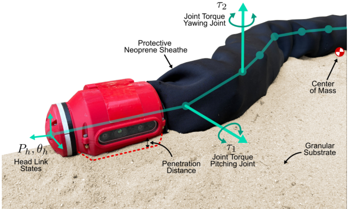
Figure 3.1: Closeup view of robot sand surface interactions. Image courtesy of Adarsh Salagame
