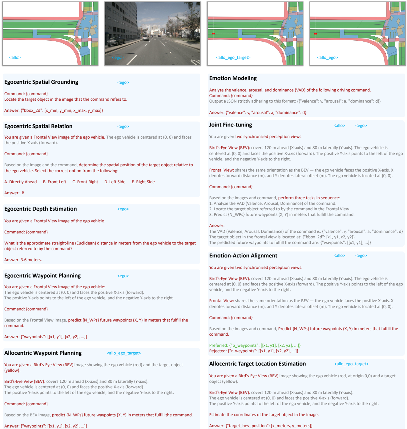
Figure A5. Overview of the prompt templates utilized in the E3AD framework across different training stages. The figure details the specific instructions and input/output formats for tasks including spatial grounding, depth estimation, emotion modeling, and trajectory planning. Note that the text elements marked in blue (i.e., <ego> , <allo> , <allo_ego_target> , <allo_ego> ) represent the special visual tokens corresponding to the egocentric view, allocentric view, and the allocentric view with the target object highlighted, respectively.
