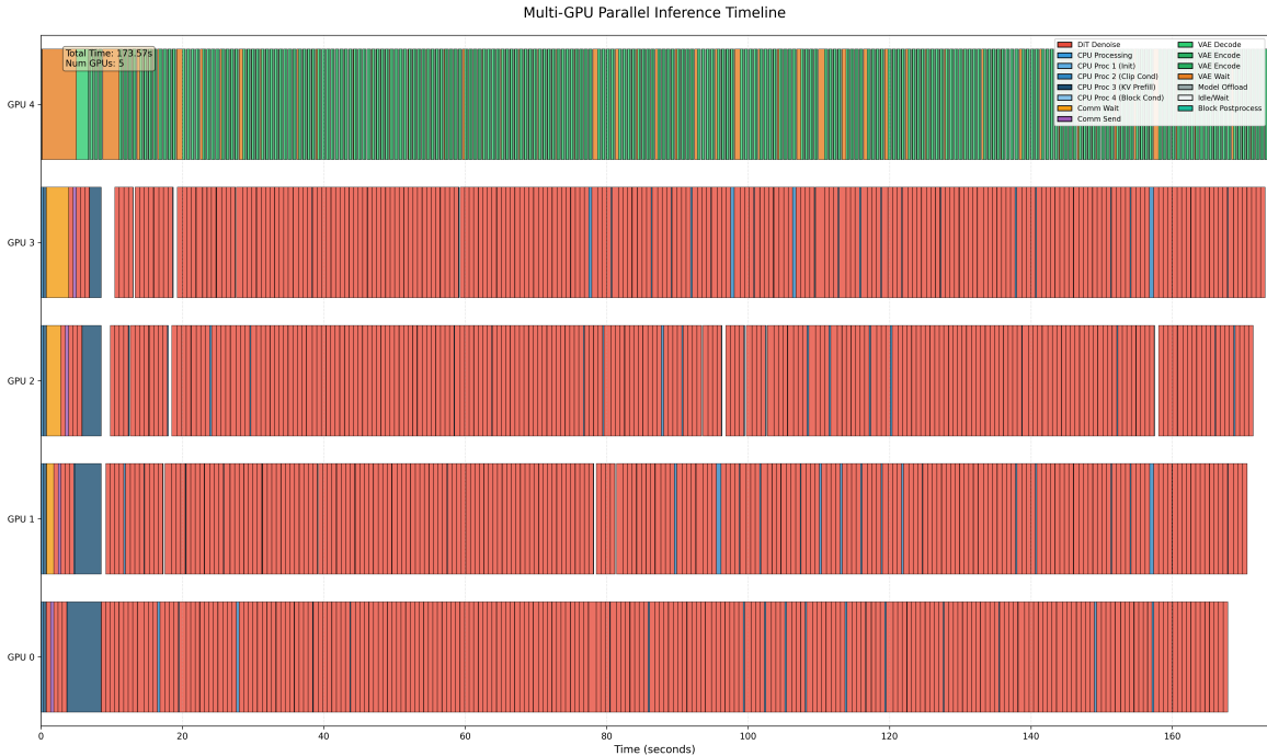
Figure 8. Multi-GPU Parallel Inference Timeline. This chart visualizes the computation and waiting periods for each GPU. The two distinct white gaps on the left represent the initial warmup phase (including the secondary warmup for AAS). Following these, the majority of the processing time is dedicated to DiT computation (shown in red ), reflecting high utilization and stable frame rates. Sporadic white gaps (idle time) appearing thereafter are present due to rate fluctuations, but their rarity ensures a negligible impact on performance.
