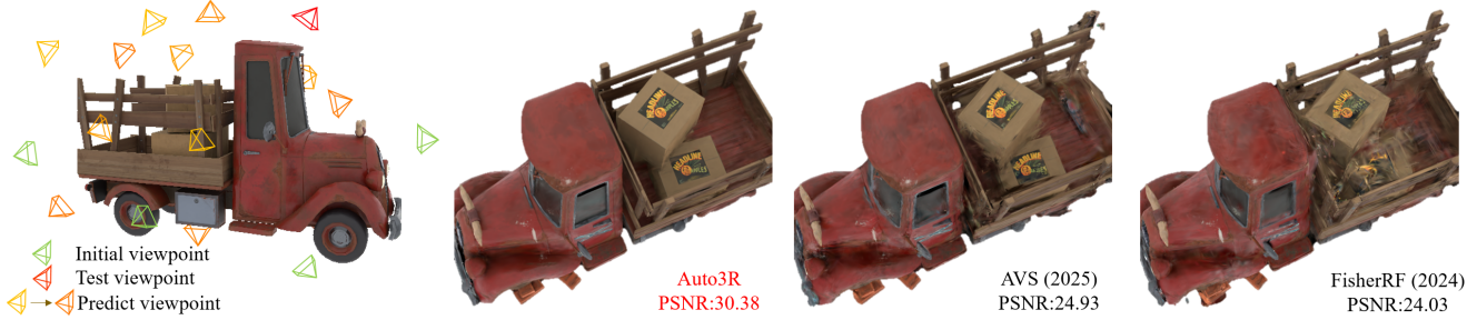
Figure 1: Left: The scanning viewpoints selected by Auto3R, exhibiting a tendency to converge toward areas with occlusion. Right: Auto3R achieves accurate reconstruction quality and significantly outperforms the state-of-the-art methods.
