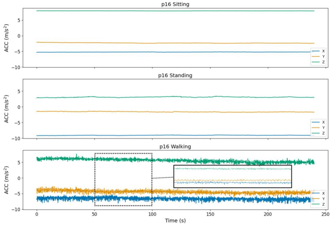
Figure 6: Triaxial ACC sensor values across physical states for subject p16. The walking state has notable oscillations compared to sitting and standing, which can be attributed to the slight swinging of the arms during gait cycles. Created in BioRender. Kaetheeswaran, J. (2025) https://BioRender.com/6j7gin4
