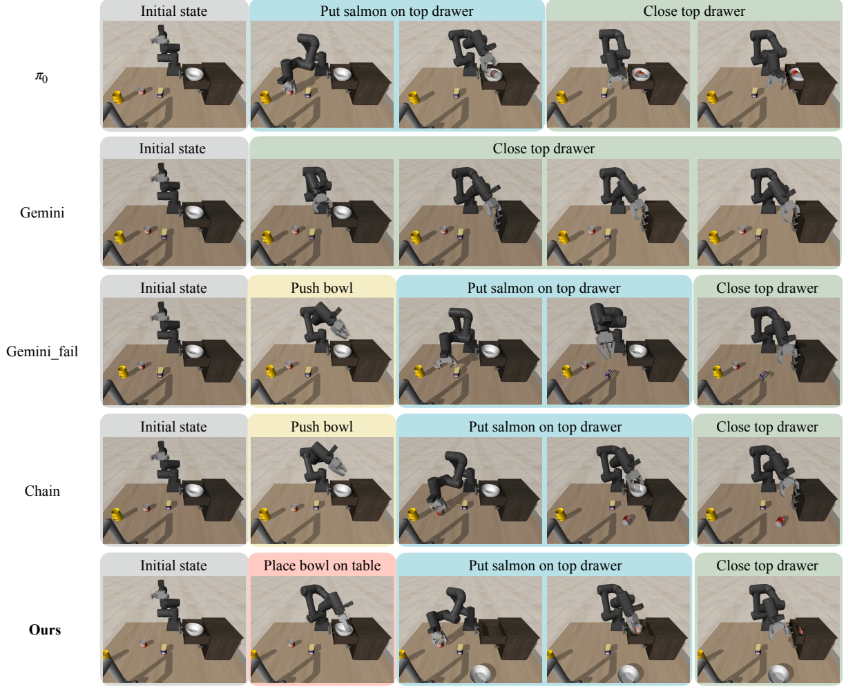
Fig. 5: Trajectory Comparison with baselines. The figure shows the trajectory generated by \pi_0 [4], VLM as system 2, i.e., Gemini-2.5-flash [49] (Gemini), and with failure examples (Gemini fail), VINE-Chain (chain), and VINE-Full (Ours) in an unseen drawer packing environment.
